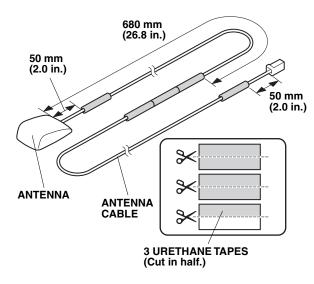
27. Wrap five of the cut pieces of urethane tape around the antenna cable at the measurements shown.
