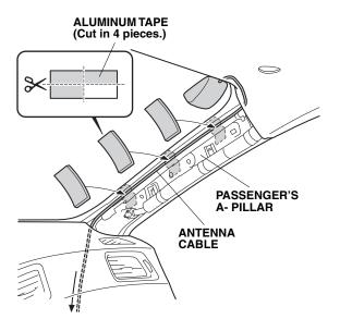
33. Route the antenna cable along the passenger's A- pillar. Using isopropyl alcohol on shop towel, clean the A-pillar where the aluminum tape will attach. Using three pieces of aluminum tape, secure the antenna cable to the A-pillar in the areas shown. NOTE: Be careful not to attach the aluminum tape over the holes in the A-pillar.
