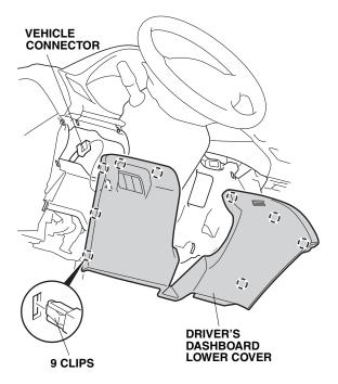
13. Remove the driver's inner dashboard trim (four clips and unplug the vehicle connector).
