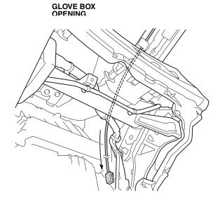
35. Using one wire tie, secure the antenna cable to the vehicle harness.
