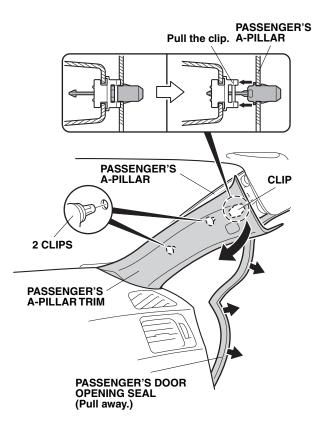
To prevent clips from falling into the body panel area, carefully insert a shop towel between the passenger's A-pillar and the passenger's A-pillar trim.
