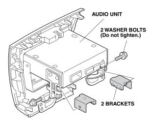
20. Install the XM radio unit onto the brackets on the audio unit with four washer bolts.
